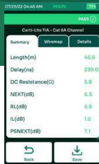
Figure 4 - Certi-Lite Autotest result can be obtained with Remote IDs. Click on Details tab to drill into each test result. Test Results can be stored in tester memory for later upload to the included PC based TestDataPro, or immediately with the included TestDataPro Cloud via wired or wireless network connection.
